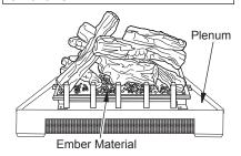
Figure 43 - Placing Ember Material on Burner
